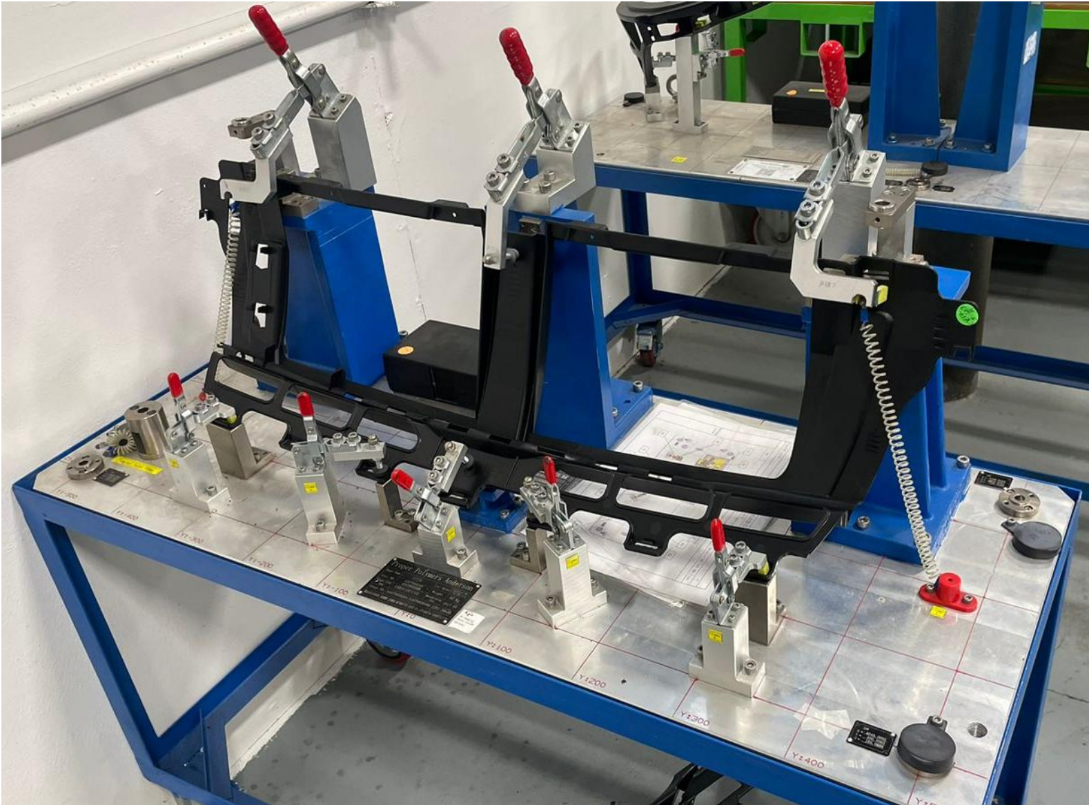
A-167-885-8205 SWITCHMOD BRACKET-CHECK FIXTURE
